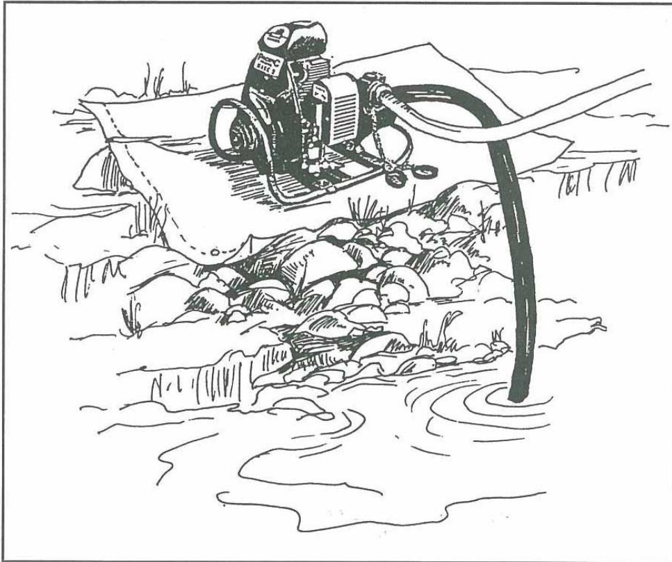
Figure 3 – Set Up Pump Close To Water Supply
