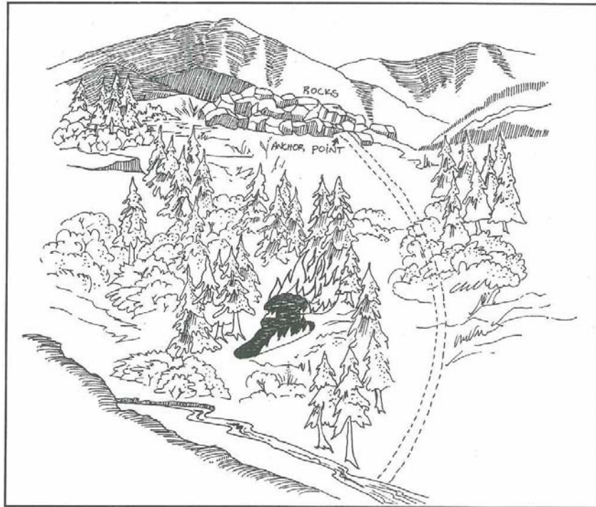
Figure 9 – Building Fireline Downhill
